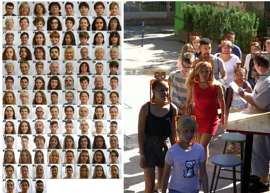
*Real-time face recognition example. On the left: single picture registration images. On the right: people are moving with normal walking speed under a 25 FPS surveillance camera. In this scenario the system can identify 96% of the people. \**
